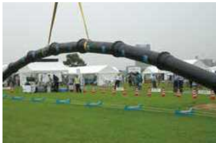
Earthquake-resistant-joint-pipes suspension demonstration
